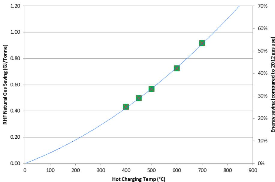
Accounting for the real situation where the furnace is charged continuously with hot billets for 60% of production time and charged from cold stock for 40%, the reduction in natural gas consumption is estimated at 0.4 GJ/tonne or 18% at a charging temperature of 450°C, as shown in . Raising the charging temperature to 700°C increases the estimated natural gas saving to 0.55 GJ/tonne or 32%.
